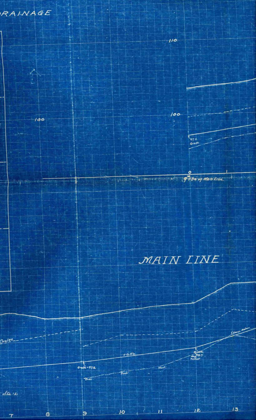
PLAT OF LOCATION OF DEAN DRA TP105 R17E MAINLINE Lacoure Late Out Elevation of Bottom of Perrime Coulee Bottom Grade Extern 33 Place 12" Tile from Sta o to Sta 12
